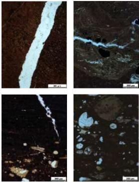
Figure 14. Thin section of silicified coal.
